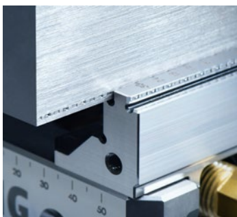
Form fit clamping with Makro•Grip®
