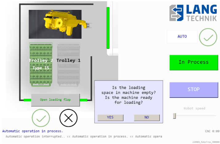
Figure 2: Part in the gripper – confirmation request
